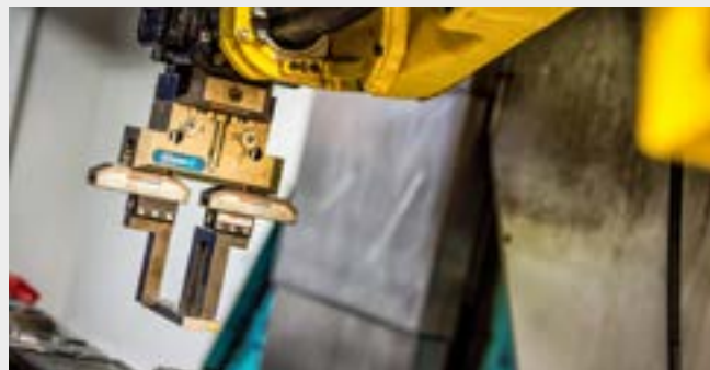
Part picking by robot
