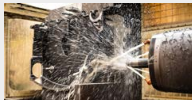
CNC Machining of cast iron saw aggregate
